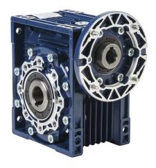
IronHorse medium-duty worm gearbox, 60:1 ratio, IEC 80B14 input, hollow, 25mm diameter output shaft, nominal 0.82hp at 1.0 SF, 1135 lb-in mechanical output torque, 63mm center distance, cast aluminum housing, top, bottom and back mount.
