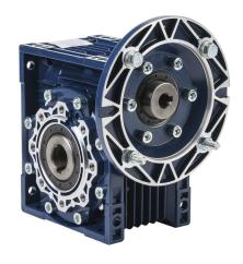
IronHorse medium-duty worm gearbox, 60:1 ratio, IEC 71B5 input, hollow, 25mm diameter output shaft, nominal 0.82hp at 1.0 SF, 1135 lb-in mechanical output torque, 63mm center distance, cast aluminum housing, top, bottom and back mount.
