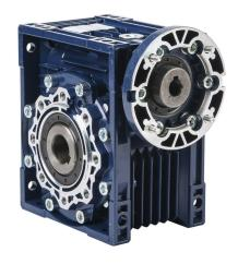
IronHorse medium-duty worm gearbox, 60:1 ratio, IEC 71B14 input, hollow, 25mm diameter output shaft, nominal 0.82hp at 1.0 SF, 1135 lb-in mechanical output torque, 63mm center distance, cast aluminum housing, top, bottom and back mount.
