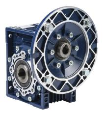
IronHorse medium-duty worm gearbox, 50:1 ratio, IEC 80B5 input, hollow, 25mm diameter output shaft, nominal 0.99hp at 1.0 SF, 1208 lb-in mechanical output torque, 63mm center distance, cast aluminum housing, top, bottom and back mount.
