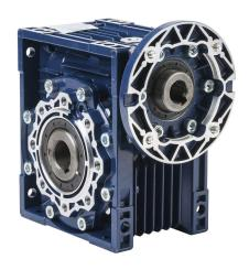
IronHorse medium-duty worm gearbox, 50:1 ratio, IEC 80B14 input, hollow, 25mm diameter output shaft, nominal 0.99hp at 1.0 SF, 1208 lb-in mechanical output torque, 63mm center distance, cast aluminum housing, top, bottom and back mount.
