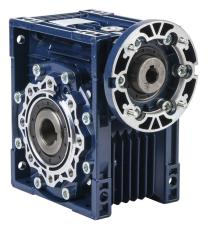
IronHorse medium-duty worm gearbox, 50:1 ratio, IEC 71B14 input, hollow, 25mm diameter output shaft, nominal 0.99hp at 1.0 SF, 1208 lb-in mechanical output torque, 63mm center distance, cast aluminum housing, top, bottom and back mount.
