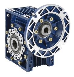
IronHorse medium-duty worm gearbox, 40:1 ratio, 56C-Face input, hollow, 1.125in diameter output shaft, nominal 1hp at 1.0 SF, 1274 lb-in mechanical output torque, 63mm center distance, cast aluminum housing, top and bottom mount.
