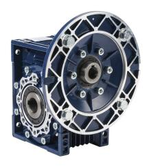
IronHorse medium-duty worm gearbox, 40:1 ratio, IEC 80B5 input, hollow, 25mm diameter output shaft, nominal 1.21hp at 1.0 SF, 1261 lb-in mechanical output torque, 63mm center distance, cast aluminum housing, top, bottom and back mount.
