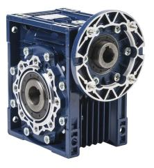
IronHorse medium-duty worm gearbox, 40:1 ratio, IEC 80B14 input, hollow, 25mm diameter output shaft, nominal 1.21hp at 1.0 SF, 1261 Ib-in mechanical output torque, 63mm center distance, cast aluminum housing, top, bottom and back mount.
