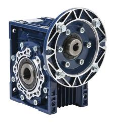
IronHorse medium-duty worm gearbox, 40:1 ratio, IEC 71B5 input, hollow, 25mm diameter output shaft, nominal 1.21hp at 1.0 SF, 1261 lb-in mechanical output torque, 63mm center distance, cast aluminum housing, top, bottom and back mount.
