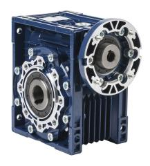
IronHorse medium-duty worm gearbox, 40:1 ratio, IEC 71B14 input, hollow, 25mm diameter output shaft, nominal 1.21hp at 1.0 SF, 1261 lb-in mechanical output torque, 63mm center distance, cast aluminum housing, top, bottom and back mount.
