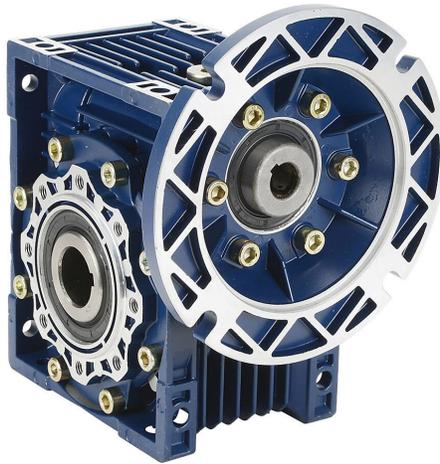
IronHorse medium-duty worm gearbox, 30:1 ratio, 56C-Face input, hollow, 1.125in diameter output shaft, nominal 1.5hp at 1.0 SF, 1416 lb-in mechanical output torque, 63mm center distance, cast aluminum housing, top and bottom mount.
