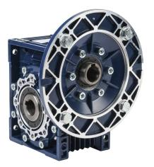
IronHorse medium-duty worm gearbox, 30:1 ratio, IEC 90B5 input, hollow, 25mm diameter output shaft, nominal 1.64hp at 1.0 SF, 1345 Ib-in mechanical output torque, 63mm center distance, cast aluminum housing, top, bottom and back mount.
