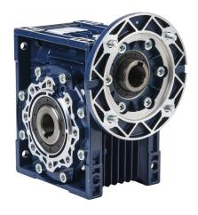
IronHorse medium-duty worm gearbox, 30:1 ratio, IEC 90B14 input, hollow, 25mm diameter output shaft, nominal 1.64hp at 1.0 SF, 1345 lb-in mechanical output torque, 63mm center distance, cast aluminum housing, top, bottom and back mount.
