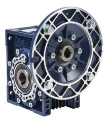
IronHorse medium-duty worm gearbox, 30:1 ratio, IEC 80B5 input, hollow, 25mm diameter output shaft, nominal 1.64hp at 1.0 SF, 1345 lb-in mechanical output torque, 63mm center distance, cast aluminum housing, top, bottom and back mount.
