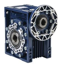
IronHorse medium-duty worm gearbox, 30:1 ratio, IEC 80B14 input, hollow, 25mm diameter output shaft, nominal 1.64hp at 1.0 SF, 1345 lb-in mechanical output torque, 63mm center distance, cast aluminum housing, top, bottom and back mount.
