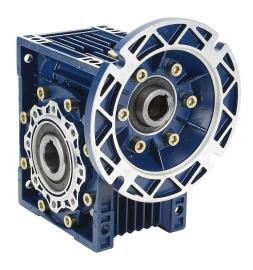
IronHorse medium-duty worm gearbox, 20:1 ratio, 145TC-Face input, hollow, 1.125in diameter output shaft, nominal 2hp at 1.0 SF, 1186 lb-in mechanical output torque, 63mm center distance, cast aluminum housing, top and bottom mount.
