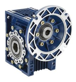
IronHorse medium-duty worm gearbox, 20:1 ratio, 56C-Face input, hollow, 1.125in diameter output shaft, nominal 2hp at 1.0 SF, 1186 lb-in mechanical output torque, 63mm center distance, cast aluminum housing, top and bottom mount.
