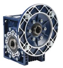
IronHorse medium-duty worm gearbox, 20:1 ratio, IEC 90B5 input, hollow, 25mm diameter output shaft, nominal 2.06hp at 1.0 SF, 1225 lb-in mechanical output torque, 63mm center distance, cast aluminum housing, top, bottom and back mount.
