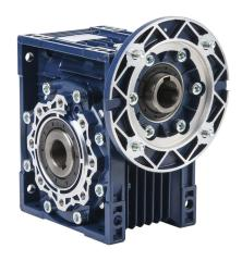
IronHorse medium-duty worm gearbox, 20:1 ratio, IEC 90B14 input, hollow, 25mm diameter output shaft, nominal 2.06hp at 1.0 SF, 1225 lb-in mechanical output torque, 63mm center distance, cast aluminum housing, top, bottom and back mount.
