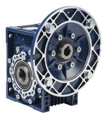
IronHorse medium-duty worm gearbox, 20:1 ratio, IEC 80B5 input, hollow, 25mm diameter output shaft, nominal 2.06hp at 1.0 SF, 1225 lb-in mechanical output torque, 63mm center distance, cast aluminum housing, top, bottom and back mount.
