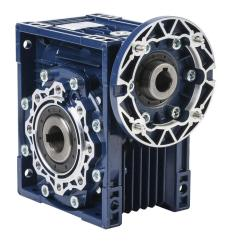
IronHorse medium-duty worm gearbox, 20:1 ratio, IEC 80B14 input, hollow, 25mm diameter output shaft, nominal 2.06hp at 1.0 SF, 1225 lb-in mechanical output torque, 63mm center distance, cast aluminum housing, top, bottom and back mount.
