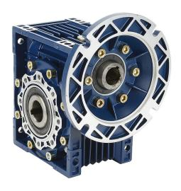
IronHorse medium-duty worm gearbox, 10:1 ratio, 145TC-Face input, hollow, 1.125in diameter output shaft, nominal 3hp at 1.0 SF, 1141 lb-in mechanical output torque, 63mm center distance, cast aluminum housing, top and bottom mount.
