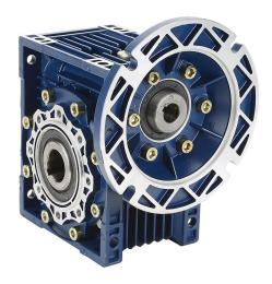
IronHorse medium-duty worm gearbox, 10:1 ratio, 56C-Face input, hollow, 1.125in diameter output shaft, nominal 3hp at 1.0 SF, 1141 lb-in mechanical output torque, 63mm center distance, cast aluminum housing, top and bottom mount.
