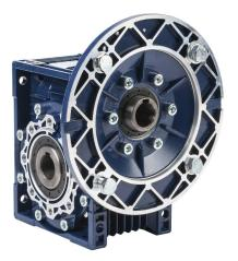
IronHorse medium-duty worm gearbox, 10:1 ratio, IEC 90B5 input, hollow, 25mm diameter output shaft, nominal 3.52hp at 1.0 SF, 1108 lb-in mechanical output torque, 63mm center distance, cast aluminum housing, top, bottom and back mount.
