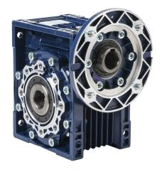
IronHorse medium-duty worm gearbox, 10:1 ratio, IEC 90B14 input, hollow, 25mm diameter output shaft, nominal 3.52hp at 1.0 SF, 1108 lb-in mechanical output torque, 63mm center distance, cast aluminum housing, top, bottom and back mount.
