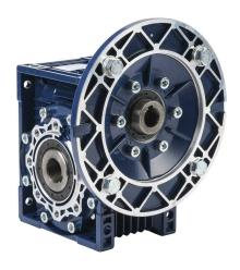
IronHorse medium-duty worm gearbox, 10:1 ratio, IEC 80B5 input, hollow, 25mm diameter output shaft, nominal 3.52hp at 1.0 SF, 1108 lb-in mechanical output torque, 63mm center distance, cast aluminum housing, top, bottom and back mount.
