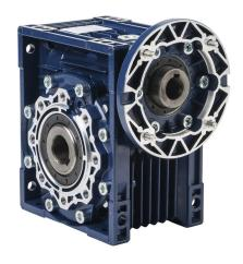
IronHorse medium-duty worm gearbox, 10:1 ratio, IEC 80B14 input, hollow, 25mm diameter output shaft, nominal 3.52hp at 1.0 SF, 1108 lb-in mechanical output torque, 63mm center distance, cast aluminum housing, top, bottom and back mount.
