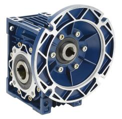
IronHorse medium-duty worm gearbox, 100:1 ratio, 56C-Face input, hollow, 1in diameter output shaft, nominal 0.25hp at 1.0 SF, 487 lb-in mechanical output torque, 50mm center distance, cast aluminum housing, top and bottom mount.
