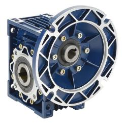
IronHorse medium-duty worm gearbox, 80:1 ratio, 56C-Face input, hollow, 1in diameter output shaft, nominal 0.33hp at 1.0 SF, 566 lb-in mechanical output torque, 50mm center distance, cast aluminum housing, top and bottom mount.
