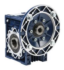
IronHorse medium-duty worm gearbox, 80:1 ratio, IEC 71B5 input, hollow, 25mm diameter output shaft, nominal 0.35hp at 1.0 SF, 546 lb-in mechanical output torque, 50mm center distance, cast aluminum housing, top, bottom and back mount.
