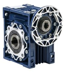
IronHorse medium-duty worm gearbox, 80:1 ratio, IEC 71B14 input, hollow, 25mm diameter output shaft, nominal 0.35hp at 1.0 SF, 546 lb-in mechanical output torque, 50mm center distance, cast aluminum housing, top, bottom and back mount.
