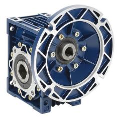
IronHorse medium-duty worm gearbox, 60:1 ratio, 56C-Face input, hollow, 1in diameter output shaft, nominal 0.33hp at 1.0 SF, 602 lb-in mechanical output torque, 50mm center distance, cast aluminum housing, top and bottom mount.
