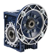
IronHorse medium-duty worm gearbox, 60:1 ratio, IEC 71B5 input, hollow, 25mm diameter output shaft, nominal 0.47hp at 1.0 SF, 605 lb-in mechanical output torque, 50mm center distance, cast aluminum housing, top, bottom and back mount.
