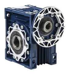
IronHorse medium-duty worm gearbox, 60:1 ratio, IEC 71B14 input, hollow, 25mm diameter output shaft, nominal 0.47hp at 1.0 SF, 605 lb-in mechanical output torque, 50mm center distance, cast aluminum housing, top, bottom and back mount.
