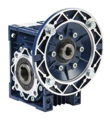
IronHorse medium-duty worm gearbox, 50:1 ratio, IEC 71B5 input, hollow, 25mm diameter output shaft, nominal 0.56hp at 1.0 SF, 647 lb-in mechanical output torque, 50mm center distance, cast aluminum housing, top, bottom and back mount.
