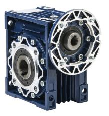
IronHorse medium-duty worm gearbox, 50:1 ratio, IEC 71B14 input, hollow, 25mm diameter output shaft, nominal 0.56hp at 1.0 SF, 647 lb-in mechanical output torque, 50mm center distance, cast aluminum housing, top, bottom and back mount.
