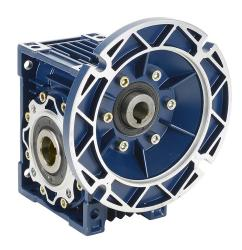
IronHorse medium-duty worm gearbox, 40:1 ratio, 56C-Face input, hollow, 1in diameter output shaft, nominal 0.75hp at 1.0 SF, 664 lb-in mechanical output torque, 50mm center distance, cast aluminum housing, top and bottom mount.
