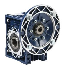
IronHorse medium-duty worm gearbox, 40:1 ratio, IEC 71B5 input, hollow, 25mm diameter output shaft, nominal 0.7hp at 1.0 SF, 689 lb-in mechanical output torque, 50mm center distance, cast aluminum housing, top, bottom and back mount.
