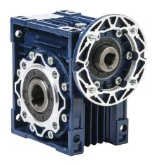
IronHorse medium-duty worm gearbox, 40:1 ratio, IEC 71B14 input, hollow, 25mm diameter output shaft, nominal 0.7hp at 1.0 SF, 689 lb-in mechanical output torque, 50mm center distance, cast aluminum housing, top, bottom and back mount.
