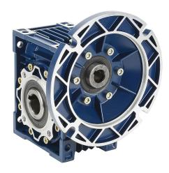
IronHorse medium-duty worm gearbox, 30:1 ratio, 56C-Face input, hollow, 1in diameter output shaft, nominal 0.75hp at 1.0 SF, 734 lb-in mechanical output torque, 50mm center distance, cast aluminum housing, top and bottom mount.
