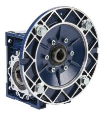
IronHorse medium-duty worm gearbox, 30:1 ratio, IEC 80B5 input, hollow, 25mm diameter output shaft, nominal 0.94hp at 1.0 SF, 740 lb-in mechanical output torque, 50mm center distance, cast aluminum housing, top, bottom and back mount.
