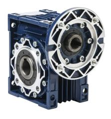
IronHorse medium-duty worm gearbox, 30:1 ratio, IEC 80B14 input, hollow, 25mm diameter output shaft, nominal 0.94hp at 1.0 SF, 740 lb-in mechanical output torque, 50mm center distance, cast aluminum housing, top, bottom and back mount.
