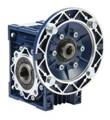
IronHorse medium-duty worm gearbox, 30:1 ratio, IEC 71B5 input, hollow, 25mm diameter output shaft, nominal 0.94hp at 1.0 SF, 740 lb-in mechanical output torque, 50mm center distance, cast aluminum housing, top, bottom and back mount.
