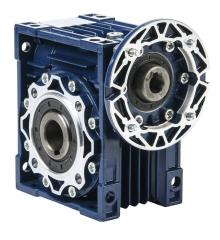
IronHorse medium-duty worm gearbox, 30:1 ratio, IEC 71B14 input, hollow, 25mm diameter output shaft, nominal 0.94hp at 1.0 SF, 740 lb-in mechanical output torque, 50mm center distance, cast aluminum housing, top, bottom and back mount.
