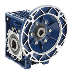
IronHorse medium-duty worm gearbox, 20:1 ratio, 56C-Face input, hollow, 1in diameter output shaft, nominal 1hp at 1.0 SF, 646 lb-in mechanical output torque, 50mm center distance, cast aluminum housing, top and bottom mount.
