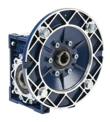
IronHorse medium-duty worm gearbox, 20:1 ratio, IEC 80B5 input, hollow, 25mm diameter output shaft, nominal 1.14hp at 1.0 SF, 656 lb-in mechanical output torque, 50mm center distance, cast aluminum housing, top, bottom and back mount.
