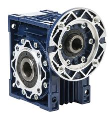
IronHorse medium-duty worm gearbox, 20:1 ratio, IEC 80B14 input, hollow, 25mm diameter output shaft, nominal 1.14hp at 1.0 SF, 656 lb-in mechanical output torque, 50mm center distance, cast aluminum housing, top, bottom and back mount.
