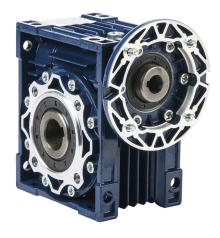
IronHorse medium-duty worm gearbox, 20:1 ratio, IEC 71B14 input, hollow, 25mm diameter output shaft, nominal 1.14hp at 1.0 SF, 656 lb-in mechanical output torque, 50mm center distance, cast aluminum housing, top, bottom and back mount.
