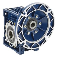
IronHorse medium-duty worm gearbox, 10:1 ratio, 56C-Face input, hollow, 1in diameter output shaft, nominal 2hp at 1.0 SF, 628 lb-in mechanical output torque, 50mm center distance, cast aluminum housing, top and bottom mount.
