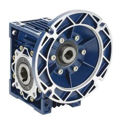
IronHorse medium-duty worm gearbox, 10:1 ratio, 56C-Face input, hollow, 1in diameter output shaft, nominal 2hp at 1.0 SF, 628 lb-in mechanical output torque, 50mm center distance, cast aluminum housing, top and bottom mount.
